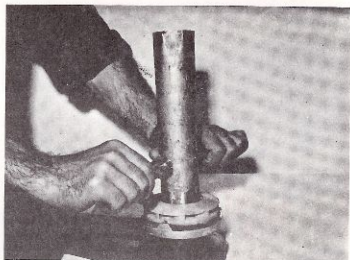
Fig. 55: Using the drive pulley clamp #2 to hold the clutch cover, loosen and remove the main retaining nut with Tool/Wrench #4.
