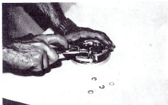
Fig. 60: The centrifugal clutch has three clutch engaging arms which open up to engage the clutch cover when the engine revolutions build up. Firstly, remove the 3 spring retaining washers with pliers.
