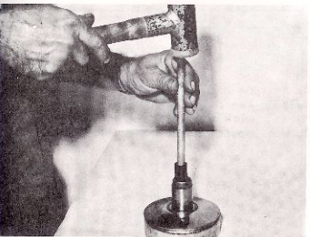
Fig. 58: Using the special tool #11, tap out the bearing and bushing.
