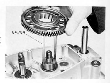
CAUTION: the freewheel hub shall be fitted so as to allow the 1st speed gear to turn free when rotated in the counter-clockwise direction.
