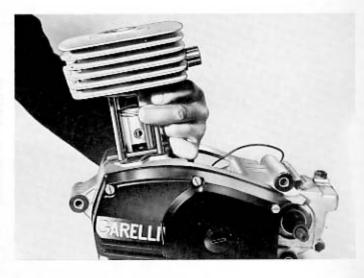
— Check that the top of the cylinder and the face of the head are clean and undamaged. Fit the gasket and the studs and place the 4 washers and nuts on the studs. Tighten the nuts gradually in a cross pattern. The final torque should be 1,5÷1,8 kpm. (in.lb. 0,084÷0,10).
