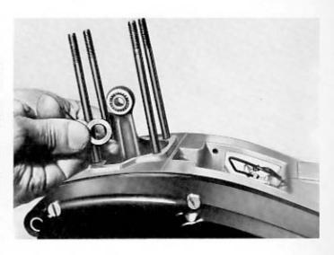
— Check that the crankcase upper face and the cylinder base are clean and free from burrs. Lightly grease a new gasket on both sides and lay it on the crankcase face. Oil the cylinder bore and the piston skirt. Lower the cylinder onto the piston with fingers compressing the rings into the bore. Make sure that the ends of the piston rings are properly fitted in position against the pegs of the rings grooves. Slide the cylinder along the 4 studs and fit it in place.
