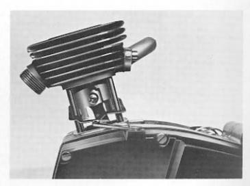
Remove the two gudgeon pin retaining circlips with the pliers.
